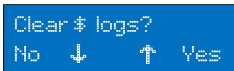
\$ is the total number of logs stored on the unit's internal memory. Press the
