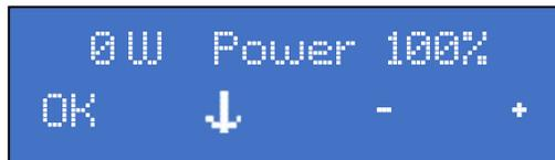
To decrease the power level setting, press and release the
