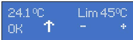
The current fluid temperature is displayed in the top left-hand corner of the screen. The current set limit temperature is displayed in the top right-hand corner of the screen.
